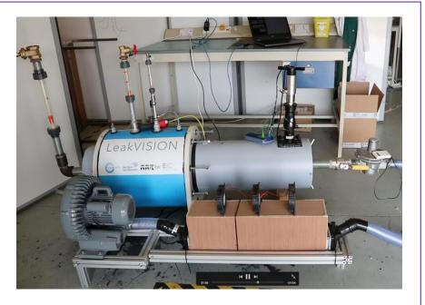
The **thermal signature of a leak** is captured and can be compared to the other areas of the pipelines to provide a **quick comparison** which highlights areas of interest for further investigation.
